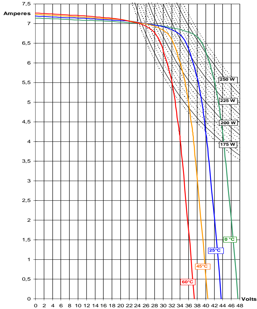
I=F(V) à E=1 \text{ kW/m}^2 , AM=1,5 as a function of the junction temperature
